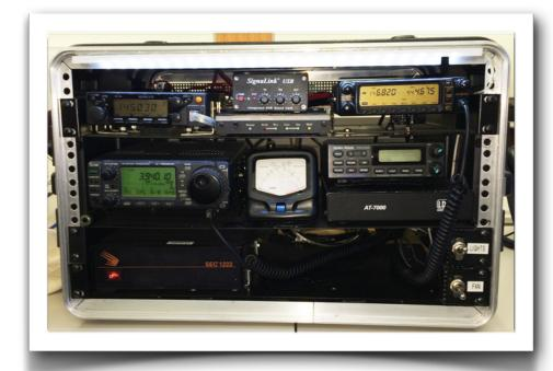
Middle Row: ICOM 706 HF Trans ceiver with an SWR meter between it and the LDG-7000 Autotuner for the 706.
